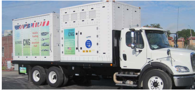
FuelMule from Ultimate CNG is a mobile, self-contained CNG station providing onsite fast-fill fuel delivery. Photo from Ultimate CNG, LLC
