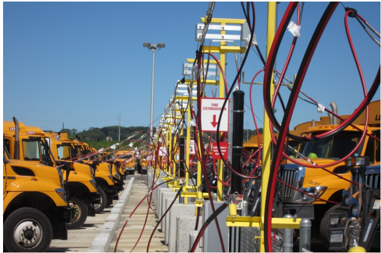
CNG vehicles using time-fill posts in Oyster Bay, New York. Photo from Greater Long Island Clean Cities, NREL 23853
